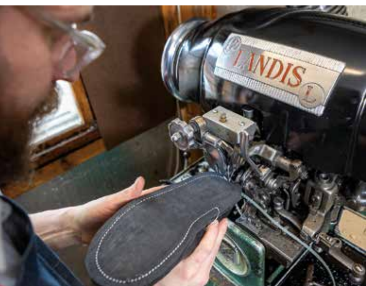
TOP LEFT: Lane-Olsen trims the leather innersole that has been temporarily tacked to the custom last. MIDDLE: Emmett Moberly-LaChance presses the midsole layer to the upper of the boot. BOTTOM: Lane-Olsen stitches the midsole layer to the upper on a 1953 Landis L curved needle stitcher using highly durable braided polyester thread. TOP RIGHT: Adam Lane-Olsen holds a new pair of custom Limmer boots.
